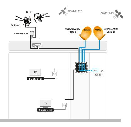
SAT. MODE = WIDEBAND SAT DC LINK = ON
