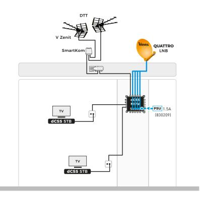
SAT. MODE = QUATTRO SAT DC LINK = ON
