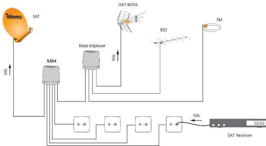
**NOTE:** To see terrestrial channels it is necessary to leave the set top box in "ON".
