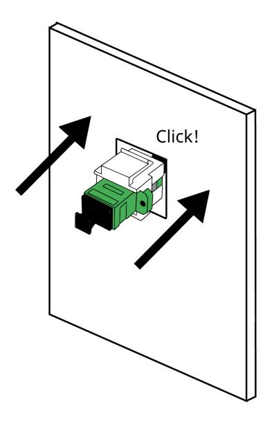
Finally, once the complete installation has been adapted, the protective caps and covers are removed and the patch cord is connected to the outlet.
