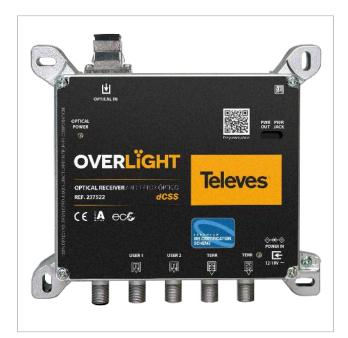
Overlight dCSS Optical Receiver with 2 dCSS/Legacy outputs For Multichoice applications, FM/DAB/UHF/SAT
