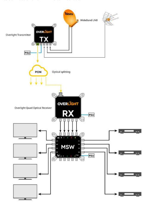
Large FTTB-type collective installation, in which the distribution of DTT and TV from 2 satellites with all its services is carried out.
