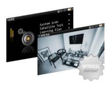
Installations of video surveillance systems are increasing. To display and monitor surveillance analog cameras, H30FLEX meters add a new software option and an USB video capture converter with Audio, Video and CVBS input connectors. H30FLEX displays NTSC and PAL video formats. The best option to verify the right functioning of the system.
