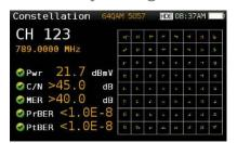
Constellation analysis is essential for determining the quality of digital signals. Constellation diagrams help detecting noise, jitter, interference and signal saturation, and all the variables that could impact signal quality, eventually leading to service suspension. By visually inspecting the size and shape of the dots in the constellation matrix, the technician will be able to easily identify the nature of the problem
