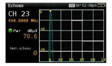
In terms of terrestial signal reception, controlling the absence of any echoes that could jeopardize reception is crucial. H30FLEX displays the echoes of the received signal, allowing the installer to minimize them for optimal signal reception.
