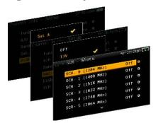
H30FLEX allows you to configure the parameters required for the reception of your satellite signal. To do this, H30FLEX allows preamplifier powering, and configuration of both DiSEqC and SCR parameters.
