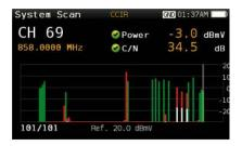
Scan each existing analogue and digital channel in real time to determine the overall system frequency response. This function leverages the location-based thresholds to clearly show whether the signal levels meet the cable systems' specifications with green, yellow and red bars. This feature provides an easy-to-understand, real-time view of the system, including the BER and MER values of the selected channel.
