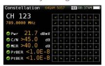
Constellation analysis is essential for determining the quality of digital signals. Constellation diagrams help detecting noise, jitter, interference and signal saturation, and all the variables that could impact signal quality, eventually leading to service suspension. By visually inspecting the size and shape of the dots in the constellation matrix, the technician will be able to easily identify the nature of the problem
