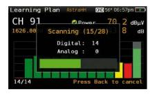
Identify the channels in your distribution with the ultra-fast Capture Plan function, and from there build your own channel plan containing only the channels you are interested in. Furthermore, each channel will be displayed on a bar chart with the appropriate colour based on the selected quality threshold.
