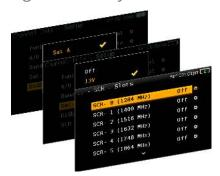
H30FLEX allows you to configure the parameters required for the reception of your satellite signal. To do this, H30FLEX allows preamplifier powering, and configuration of both DiSEqC and SCR parameters.
