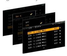
H30Evolution allows you to configure the parameters required for the reception of your satellite signal. To do this, H30Evolution allows pre-amplifier powering, and configuration of both DiSEqC and SCR parameters.
