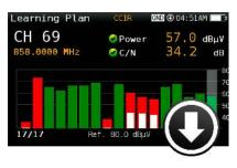
The meter automatically detects if there is a new software version when it connects to the internet (WiFi, Ethernet). To notify that new software is available, an icon in the upper right part is activated without interrupting the user's work. The system update can be accessed on the settings menu.
