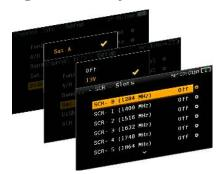
H30Evolution allows you to configure the parameters required for the reception of your satellite signal. To do this, H30Evolution allows pre-amplifier powering, and configuration of both DiSEqC and SCR parameters.
