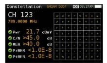
Constellation analysis is essential for determining the quality of digital signals. Constellation diagrams help detecting noise, jitter, interference and signal saturation, and all the variables that could impact signal quality, eventually leading to service suspension. By visually inspecting the size and shape of the dots in the constellation matrix, the technician will be able to easily identify the nature of the problem
