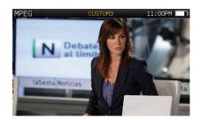
Do you wish to know the contents offered on a DIGITAL channel? H30Evolution function MPEG will tell you. In addition to channel services display, you will get their key parameters: Service name, PID, resolution, audio types and figures, and NIT. A valuable help when troubleshooting your encoder configuration.
