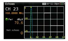
In terms of terrestial signal reception, controlling the absence of any echoes that could jeopardize reception is crucial. H30Evolution displays the echoes of the received signal, allowing the installer to minimize them for optimal signal reception.
