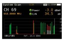
Scan each existing analogue and digital channel in real time to determine the overall system frequency response. This function leverages the location-based thresholds to clearly show whether the signal levels meet the cable systems' specifications with green, yellow and red bars. This feature provides an easy-to-understand, real-time view of the system, including the BER and MER values of the selected channel.
