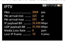
Provides demodulation and analysis of IPTV streams (both Unicast and Multicast), display both total bitrate and bitrate for each service. The relevant information for each service is: SID, VPID, AID, video profile, bit rate for both audio and video.
