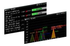
This functionality allows a full analysis of the Wi-Fi band for automatic detection of all networks. Each of them is identified by name, and the power of the signal at the access point is also displayed. Two display modes are provided for the user to choose. The "list" mode provides a list of the detected networks with the associated data and power, while the "map" mode represents them on a dual-axis map: power vs. frequency.
