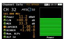
H30Evolution provides a deep and detailed analysis of ATSC 3.0 signals. It also provides full analysis of ATSC1.0 and QAM signals, with the ability to decode and display the video and audio parameters of received RF signals.
