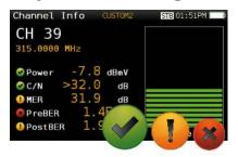
Reduce installation mistakes with the on-screen Pass/Fail indicators, a graphical tool that helps and speeds up the interpretation of measurement results. Different thresholds are available depending on the network area to be analyzed: headend, multi-band amplifiers, bridging connection, connection records, user home, etc. Besides the pre-set values, you will be able to customize your own threshold values.
