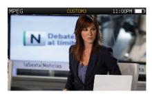
Do you wish to know the contents offered on a DIGITAL channel? H30Evolution function MPEG will tell you. In addition to channel services display, you will get their key parameters: Service name, PID, resolution, audio types and figures, and NIT. A valuable help when troubleshooting your encoder configuration.
