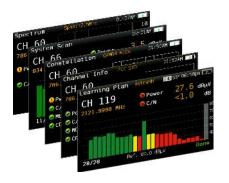
A full range of functionalities such as Single-channel measurements, Constellation diagram, Spectrum analyzer, Service identification, Data logs, Channel plan auto-learning, and more.
