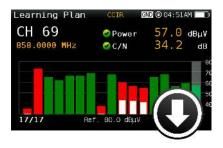
The meter automatically detects if there is a new software version when it connects to the internet (Wi-Fi, Ethernet). To notify that new software is available, an icon in the upper right part is activated without interrupting the user's work. The system update can be accessed on the settings menu.
