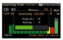
Identify the channels in your distribution with the ultra-fast Capture Plan function, and from there build your own channel plan containing only the channels you are interested in. Furthermore, each channel will be displayed on a bar chart with the appropriate colour based on the selected quality threshold.
