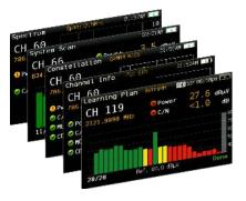
A full range of functionalities such as Single-channel measurements, Constellation diagram, Spectrum analyser, Service identification, Data logs, Channel plan auto-learning, and more.
