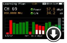
The meter automatically detects if there is a new software version when it connects to the internet (WiFi, Ethernet). To notify that new software is available, an icon in the upper right part is activated without interrupting the user's work. The system update can be accessed on the settings menu.
