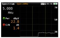
The capacity of the meter to measure the backwards channel from 5 MHz is very useful for cable installation technicians. By displaying the signal in the spectrum, measuring power and C/N, it is possible to ensure a good status and quality of the upload data transmitted on this bandwidth.
