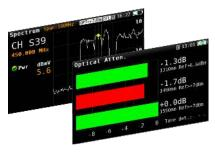
This equipment is fitted with an optical receiver (selective or nonselective options) allowing to measure power and attenuation at wavelengths of 1310nm, 1490nm and 1550nm. Combining the selective option with the triple-light generator (OPS3L) is the right choice to certify many optical infrastructures.
