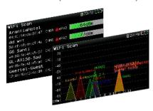
This functionality allows a full analysis of the Wi-Fi band for the automatic detection of all the networks. Each of them is identified by name, and the power of the signal at the access point is also displayed. Two display modes are provided for the user to choose. The "list" mode provides a list of the detected networks with the associated data and power, while the "map" mode represents them on a dual-axis map: power vs. frequency.
