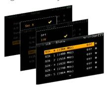
H30Crystal allows you to configure the parameters required for the reception of your satellite signal. To do this, H30Crystal allows preamplifier powering, and configuration of both DiSEqC and SCR parameters.
