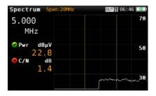
The capacity of the meter to measure the backwards channel from 5 MHz is very useful for cable installation technicians. By displaying the signal in the spectrum, measuring power and C/N, it is possible to ensure a good status and quality of the upload data transmitted on this bandwidth.
