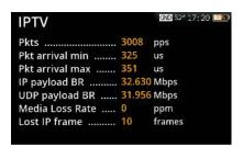
Allows the demodulation and analysis of IPTV streams (both Unicast and Multicast), not only through video display but also by displaying the total bitrate and bitrate for each service. The relevant information for each service is already given: SID, VPID, AID, video profile, bit rate for both audio and video.
