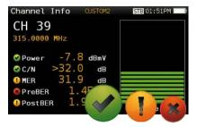
Reduce installation mistakes with the on-screen Pass/Fail indicators, a graphical tool that helps and speeds up the interpretation of measurement results. Different thresholds are available depending on the network area to be analysed: headend, multi-band amplifiers, bridging connection, connection records, user home, etc. Besides the pre-set values, you will be able to customize your own threshold values.
