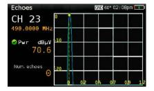
In terms of terrestial signal reception, controlling the absence of any echoes that could jeopardize reception is crucial. H30Crystal displays the echoes of the received signal, allowing the installer to minimize them for optimal signal reception.
