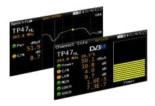
This functionality for DVB-S/S2 allows the complete analysis of a satellite channel in any frequency within the 250 MHz to 2300 MHz range. Thus, the meter can be directly connected to any output of a LNB Wideband (2 outputs: Vertical and Horizontal)
