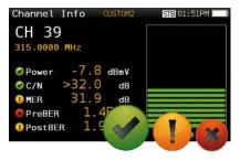
Reduce installation mistakes with the on-screen Pass/Fail indicators, a graphical tool that helps and speeds up the interpretation of measurement results. Different thresholds are available depending on the network area to be analysed: headend, multi-band amplifiers, bridging connection, connection records, user home, etc. Besides the pre-set values, you will be able to customize your own threshold values.
