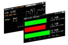
This equipment is fitted with an optical receiver (selective or nonselective options) allowing to measure power and attenuation at wavelengths of 1310nm, 1490nm and 1550nm. Combining the selective option with the triple-light generator (OPS3L) is the right choice to certify many optical infrastructures.
