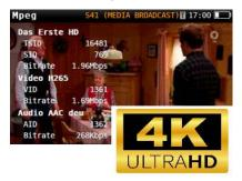
This functionality supports HEVC H.265 new compression format and allows to display video signals with a maximum Full HD resolution (1920 x 1080). Information can be displayed both on the meter screen\* or on the mobile device (multiscreen mode) as long as your hardware is H.265 compatible (usually a smartphone, tablet or PC). (\*) Optional function: Ref. 593252
