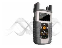
Designed to instantly obtain all the information about the signal in real time, it is a true milestone in field work. H30Crystal provides the required accuracy and speed to detect minor transient radiation, or spurious signals that could affect the system during signal reception.
