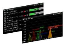
This functionality allows a full analysis of the Wi-Fi band for the automatic detection of all the networks. Each of them is identified by name, and the power of the signal at the access point is also displayed. Two display modes are provided for the user to choose. The "list" mode provides a list of the detected networks with the associated data and power, while the "map" mode represents them on a dual-axis map: power vs. frequency. (\*) Optional feature: Ref. 593250
