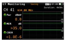
The H30+ Long Term Monitoring Function allows the automatic monitoring of the selected channel. Once the time interval between two consecutive measurements has been selected, the H30+ will automatically take all the measurements of the channel selected and store them in memory.
