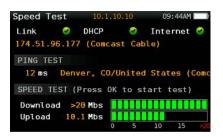
Need a quick check of your data network at the headend or at a customer's unit? The H30+'s IP Speed Test allows you to check your basic network performance parameters so you don't need to get your laptop out. This includes your upload and download speeds as well as your ping times and lost packets statistics.
