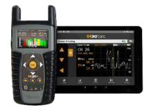
The H30+ multiscreen system allows you to display the meter's screen on your smartphone or tablet to wirelessly control the meter or just for the sake of working with a larger screen.
