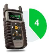
High quality Li-Ion batteries, in conjunction with our advanced low power consumption technology, provide enough juice for even the largest jobs. One hour of fast charging will provide almost three hours of extended operation.
