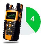
High quality Li-Ion batteries, in conjunction with our advanced low power consumption technology, provide enough juice for even the largest jobs. One hour of fast charging will provide almost three hours of extended operation.
