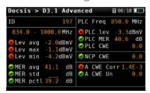
This function displays all the measurements for the DOCSIS OFDM channel. In addition to MER and level measurements, it also displays all the PLC and NCP measurements.
