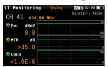
The H30D+ Long Term Monitoring Function allows the automatic monitoring of the selected channel. Once the time interval between two consecutive measurements has been selected, the H30D+ will automatically take all the measurements of the channel selected and store them in memory.
