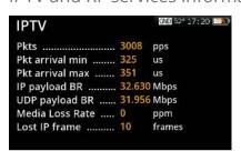
Allows the demodulation and analysis of IPTV streams (both Unicast and Multicast), not only through video display but also by displaying the total bitrate and bitrate for each service. The relevant information for each service is already given: SID, VPID, AID, video profile, bit rate for both audio and video.
