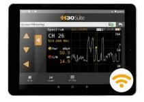
Equipped with Wireless connectivity, the equipment allows secure access through an Android or iOS device, or a PC. The web management application H30Suite (ref. 100016) may be used to check and export stored measurements, access to quality profiles, meter settings cloning, meter registration through a friendlier interface or real-time consultation of the user manual.
