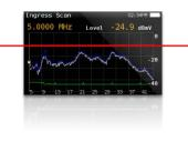
Help identify reverse path problems before your customers are affected. Poorly shielded coaxial cable and faulty terminations are important sources of ingress noise, which can easily add up in the return due to the large number of subscriber-generated signals that are sent back to the headend. The combined and amplified interference is often responsible for service disruption, so having a good reverse path ingress scan tool is always a must.
