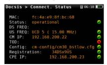
Obtain a step-by-step indication of a pass/fail test, as the modem finds, connects, and registers to a headend (CMTS), and also obtains critical parameters in the process. Confirm that the modem first finds the downstream channel and, right after that, the upstream channel. Later obtain the configuration as the DHCP address server, TOD server time, the complete configuration file and the registration information.
