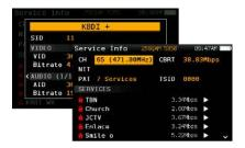
Do you want to know what program content is on that QAM channel? The H30D+'s Service Info feature will tell you. In addition to the short description of the service, you will get the important parameters including the NIT, PAT, and TSID for the channel, and for the individual service you will get the SID and the PID, encode type, resolution, and bitrate for both the audio and video, all of which greatly help when troubleshooting your encoder configuration.
