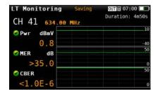
The H30D+ Long Term Monitoring Function allows the automatic monitoring of the selected channel. Once the time interval between two consecutive measurements has been selected, the H30D+ will automatically take all the measurements of the channel selected and store them in memory.
