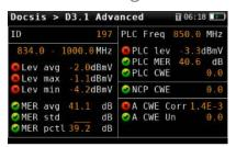
This function displays all the measurements for the DOCSIS OFDM channel. In addition to MER and level measurements, it also displays all the PLC and NCP measurements.
