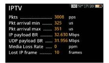
Allows the demodulation and analysis of IPTV streams (both Unicast and Multicast), not only through video display but also by displaying the total bitrate and bitrate for each service. The relevant information for each service is already given: SID, VPID, AID, video profile, bit rate for both audio and video.
