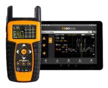
The H30D+ multiscreen system allows you to display the meter's screen on your smartphone or tablet to wirelessly control the meter or just for the sake of working with a larger screen.
