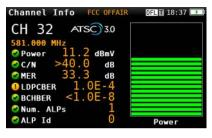
H30D+ provides a deep and detailed analysis of ATSC 3.0 signals. It also provides full analysis of ATSC 1.0 and QAM signals, with the ability to decode and display the video and audio parameters of received RF signals.
