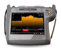
Professional spectrum analyzer with ultra-fast digital processing (sweep time < 10 ms) and high dynamic range (> 50 dB). Equipped with advanced functions for the detection and analysis of signals in the 5 MHz to 3,300 MHz (waterfall, event triggers, markers, user configurable RBW and VBW, etc.).
