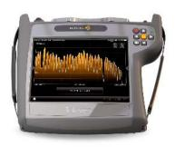
By just connecting the RF cable to your MOSAIQ6 you will find out which satellite your antenna is pointing to. Without the need for previous checks or configurations.
