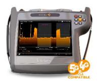
It analyses the impact of the LTE signal on the DTT channels, and detects whether the use of filters is required. Furthermore, it allows spectrum simulation upon the introduction of the LTE filter recommended by the meter itself.
