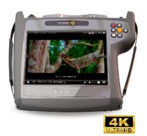
The MOSAIQ6 supports the HVEC H.265 video compression format with a maximum resolution of 4K - UHD ( $3840 \times 2160$ ) as well as the HDR colour coding standards.
