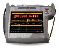
Reduce installation mistakes with the on-screen Pass/Fail indicators, a graphical tool that helps and speeds up the interpretation of measurement results. Different thresholds are available depending on the network area to be analyzed: headend, multi-band amplifiers, bridging connection, connection records, user home, etc. Besides the pre-set values, you will be able to customize your own threshold values.
