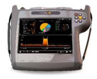
This function allows you to demodulate a DAB channel, providing signal quality measurements such as MER and CBER, and comprehensive information about the services delivered: Radio info: (Ensemble, PTY, Service, Mode, Audio- , bit rate audio). It allows power measuring between 20 dBµV and 128 dBµV, C/N and MER for this type of signals.
