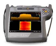
Signal levels turn into colours and are represented on the time axis (see figure). The perfect tool for short signal interference or fading analysis, which observation would be difficult by only resorting to the spectrum.
