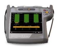
Once the optical fibre input enabled, and thanks to the optical receiver (whether selective or not), optical attenuation measuring can proceed for three wavelengths (1310 nm, 1490 nm, and 1550nm) and their powers, as does RFoG installation analysis.
