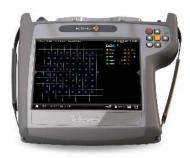
The constellation diagram is essential to help detect the presence of noise, phase jitter, interference and other potential problems that could impact the signal quality by reducing MER. The echo graphic display allows echo detection in DVB-T/T2 terrestrial signal reception, which could severely degrade BER measurement.
