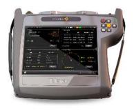
This functionality offers several control utilities and network monitoring, which can be displayed in mosaic mode. All network information at the same time, on a single screen (IP, DNS, gateway, connection mode...).
