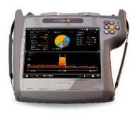
This function allows you to demodulate a DAB channel, providing signal quality measurements such as MER and CBER, and comprehensive information about the services delivered: Radio info: (Ensemble, PTY, Service, Mode, Audio- , bit rate audio). It allows power measuring between 20 dBµV and 128 dBµV, C/N and MER for this type of signals.
