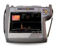
This function allows you to display and measure the analogue TV channels still used in transmodulator-based TV systems. It allows the measuring of signal levels between 20 dB $\mu$ V and 128 dB $\mu$ V, C/N up to 52 dB, and V/A up to 30 dB.
