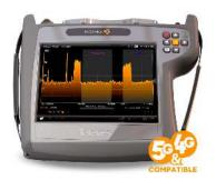
It analyses the impact of the LTE signal on the DTT channels, and detects whether the use of filters is required. Furthermore, it allows spectrum simulation upon the introduction of the LTE filter recommended by the meter itself.
