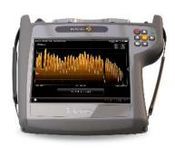
By just connecting the RF cable to your MOSAIQ6 you will find out which satellite your antenna is pointing to. Without the need for previous checks or configurations.
