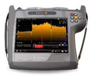
Professional spectrum analyzer with ultra-fast digital processing (sweep time < 10 ms) and high dynamic range (> 50 dB). Equipped with advanced functions for the detection and analysis of signals in the 5 MHz to 3,300 MHz (waterfall, event triggers, markers, user configurable RBW and VBW, etc.).
