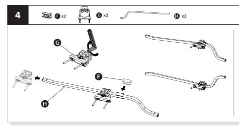
Place the plastic spacers **(F)** on the support braces (H), closer to the curved part of the support brace as indicated. Slide the mounting clamp assemblies **G** on the support braces starting from the support brace end that is not curved and tighten the bolts loosely once in place over the plastic spacers **(F)**, as they will be fully tightened later.
