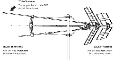
Ensure that the longest boom is assembled to be the top of the antenna as shown in the diagram. The tilt/elevation adjustment on the mounting clamps, shown in the diagram, allows for adjustment of the vertical angle of the antenna as needed for optimum reception. Starting from a horizontal position, use the mounting clamps to adjust tilt/elevation if needed for better antenna adjustment and to aim over nearby obstacles.
