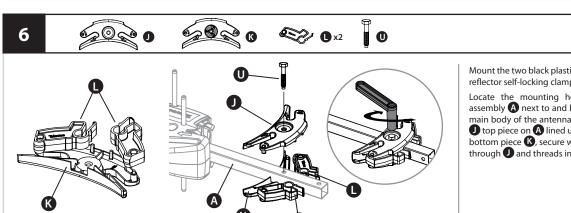
Mount the two black plastic locks on the first rear reflector self-locking clamp **(K)** bottom piece.
