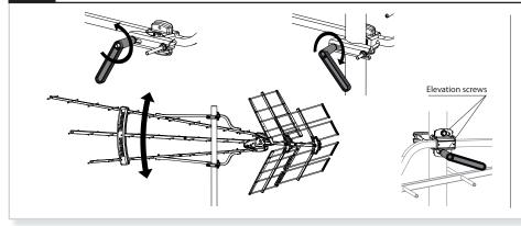
Release the shackles from the mast clamps **6** by removing and saving the shackle and nuts. Place the antenna assembly on the mast (not included) and proceed to replace the shackles and tighten the nuts to attach the assembly to the mast.
