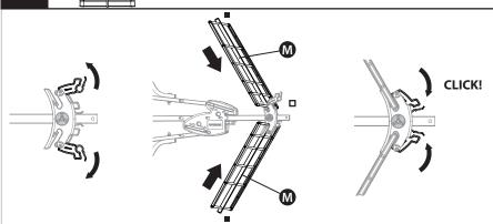
Place the **M** UHF reflectors (two pieces, one top and one bottom) in the self-locking clamp completed on step 6 by inserting the end of the receptor without the grey plastic cap on it and with the black plastic locking mechanism in an upward position
