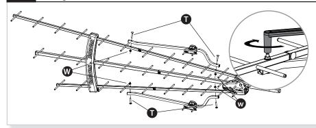
Place the support brace assemblies completed on step 4 on directors B1 (top) and B3 (bottom) as indicated, and attach them with two pieces of carriage bolt **1** and nut **W** per each support brace. Make sure the U-bolt side of the mounting clamps both are located on the left side of the support braces looking at it from a rear view. Line up the clamps so that they are ready for mounting once assembly is complete.
